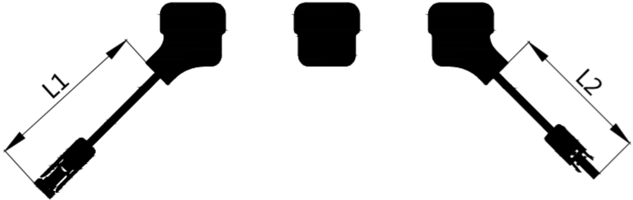
Figure 11 (2): The half-cut module/SWAN bifacial module junction box
