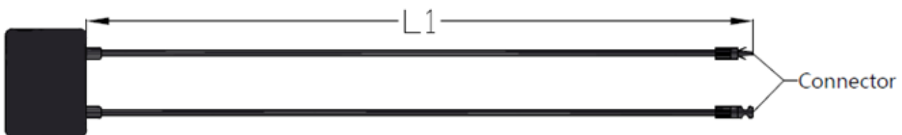
Figure 11 (1): The full module junction box
